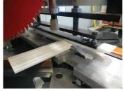
Quick, no-tool change-over for varying material widths.
